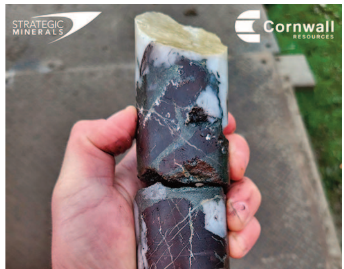
Core sample from Redmoor, showing an amazing 18.9% WO 3
